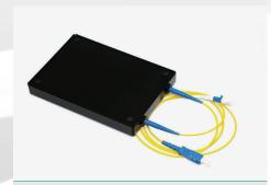
OTDR LAUNCH BOX An Optical Time Domain Reflectometer (OTDR) launch cable connects the OTDR to the fiber link under test. Its function is to overcome the "Dead Zone" which is caused by the near end reflection at the OTDR connector interface. Using a launch cable enables an accurate near end measurement of the input connector of the fiber link under test.
