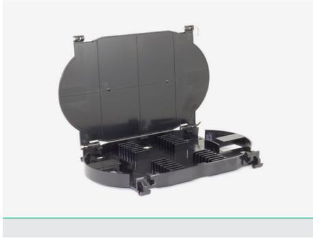
**SPLICE TRAYS** Splice trays organize and provide protection for fusion and mechanical splicing methods. They can be used indoor or outdoor with loose-tube or tight-buffered cables. Made of lightweight, durable plastic they are stocked in 12 and 24-fiber versions and include attachment points for strain relief.
