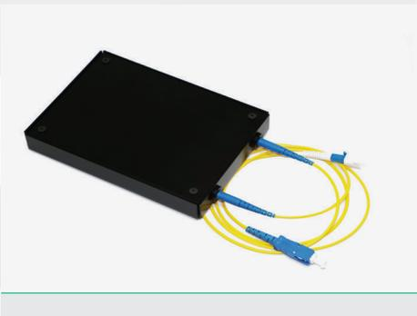
**OTDR LAUNCH BOX** An Optical Time Domain Reflectometer (OTDR) launch cable connects the OTDR to the fiber link under test. Its function is to overcome the "Dead Zone" which is caused by the near end reflection at the OTDR connector interface. Using a launch cable enables an accurate near end measurement of the input connector of the fiber link under test.
