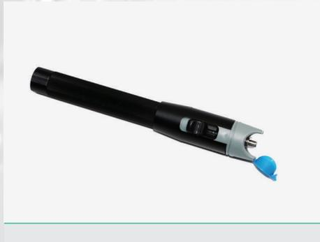
**VISUAL FAULT LOCATOR** LITRA MFG offers a Visual Fault Locator (VFL) based on a high power red laser emitting at a wavelength of 650nm. The VFL-30-U is a compact, pen-shaped VFL with an optical output of 30mW. Applications include: Location of fiber bends or breaks, determination of fiber connector and splice failures, identification and tracing of fibers between patch panels. Operation in continuous wave or pulsed mode enables simplification of the trouble-shooting process.
